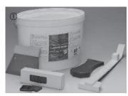
Installation tools: Special tapping block, distance spacers, professional pull tool, flexible glue, notched applicator D, pencil, pocket rule.
